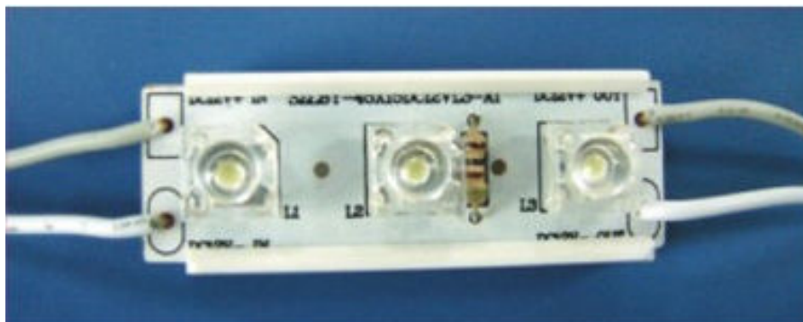
Model: Non-waterproof Super Flux Module 3-LED
